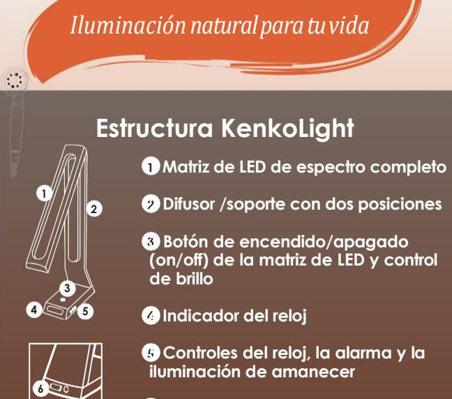
The diagram illustrates the six main components of the KenkoLight:
